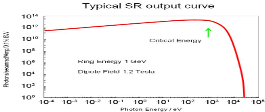
The critical energy (or frequency) is defined as the energy where the integrated spectral energy distribution is separated into two equal parts.
